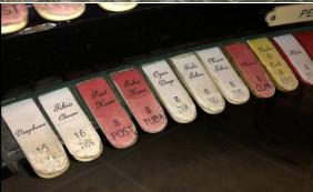
New console bolsters with SAMs. All stop tabs have had the old paper removed and cleaned.
